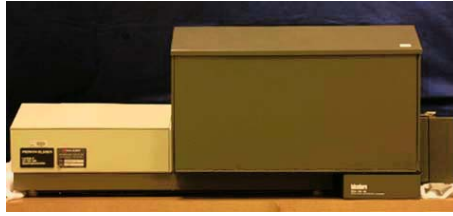
Fig. 1. Example of a Spectrophotometer. Perkin-Elmer Lambda-19 Spectrophotometer. Spectral range 250-2500 nm with a 1.00 nm slit width ( www.grc.nasa.gov/WWW/epbranch/OpticalProps/lambda.htm )
