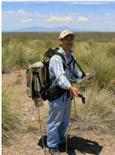
Fig. 2. Example of a field spectroradiometer. Analytical Spectral Devices FieldSpec ProFR, spectral range 350-2500 nm with a 3-10 nm slit width. ( www.asdi.com/products.specifications-FSP.asp )
